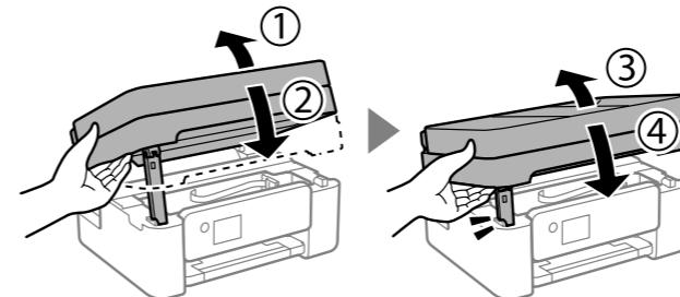
The unit must be closed completely before it can be opened again.
